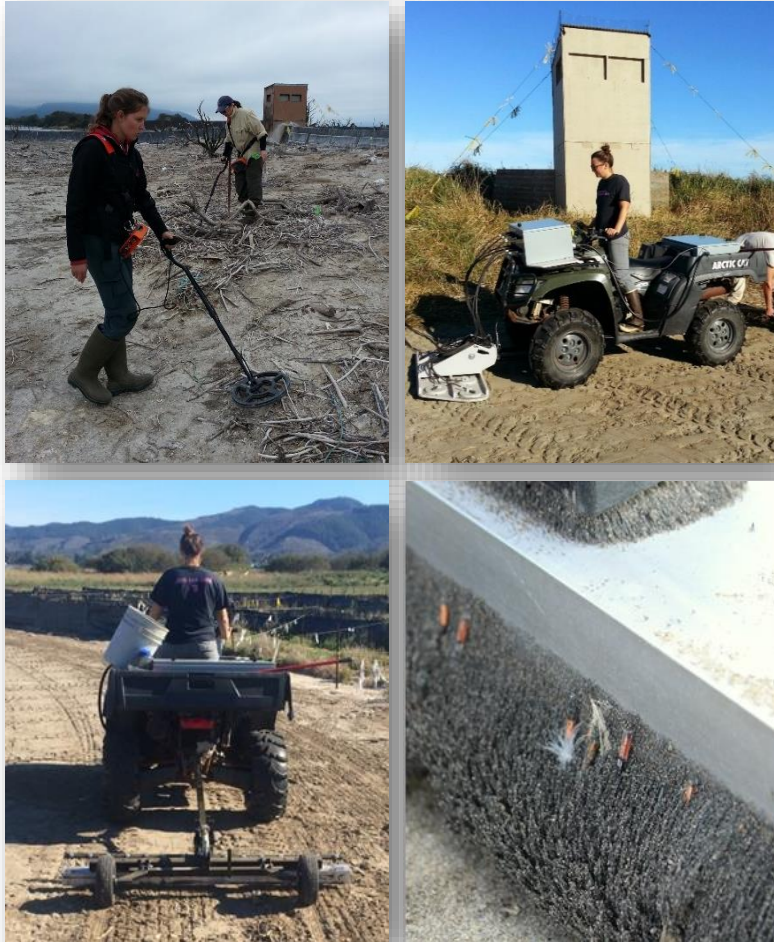
Figure 1: PIT tag detection equipment used on East Sand Island in 2015 included a hand-held portable system (top left), an eight coil flat-plate system attached to an ATV (top right), and a towable sweeper magnet attached to an ATV (bottom right and left).
